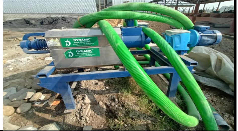
Fluid extraction from the cow dung to prepare dry manure (one of the innovation)
