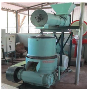
Figure 27: Machine for making straw based pellets
