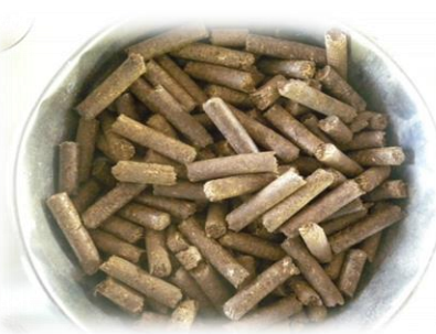
Figure 28: Straw based pellets
