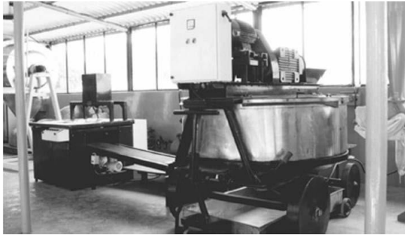
Figure 21: UMMB plant developed by NDDB in India
