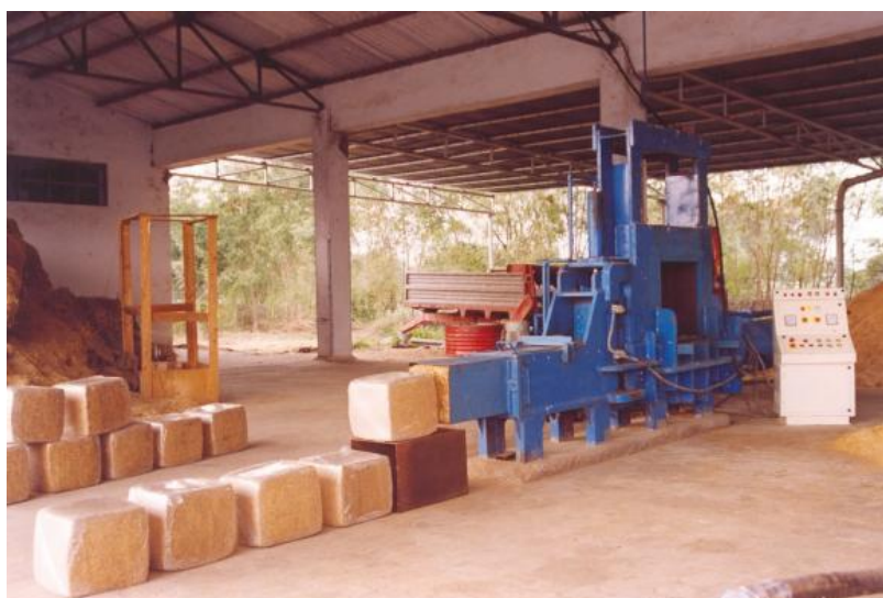
Figure 30: Block making machine
