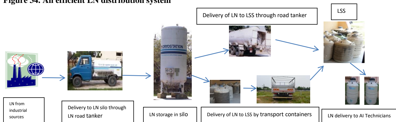
Figure 34. An efficient LN distribution system
